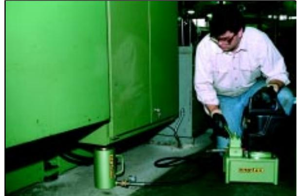
The problem was to reposition machine centers without disrupting production. "Using Simplex RLR Series cylinders and a PE70 series **Suc-O-Matic** pump, we rearranged our shop floor in one day." The low closed height and longer strokes eliminated extra jacking & blocking procedures, and the Simplex Suc-O-Matic retracted load return cylinders effortlessly.
