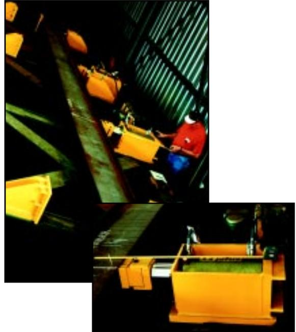
A heavy steel fabricator uses Simplex RDA10012 double acting cylinders to form large sections of I-beam. "The Simplex cylinders and pumps allow us to bend the beams to precise radiuses."
